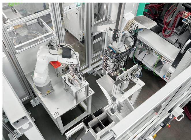
**Fig. 3.** Stations in automated production: removing the molded parts and inserting bushings into the mold (left); next to that: a bird's-eye view of the Kuka placement robot and the Multilift Robot system in action.
