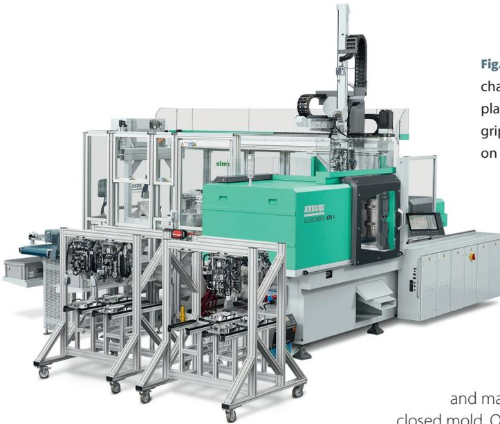
**Fig. 2.** To enable a quick changeover, the transfer plates and the matching grippers are available on two trolleys. © Arburg
